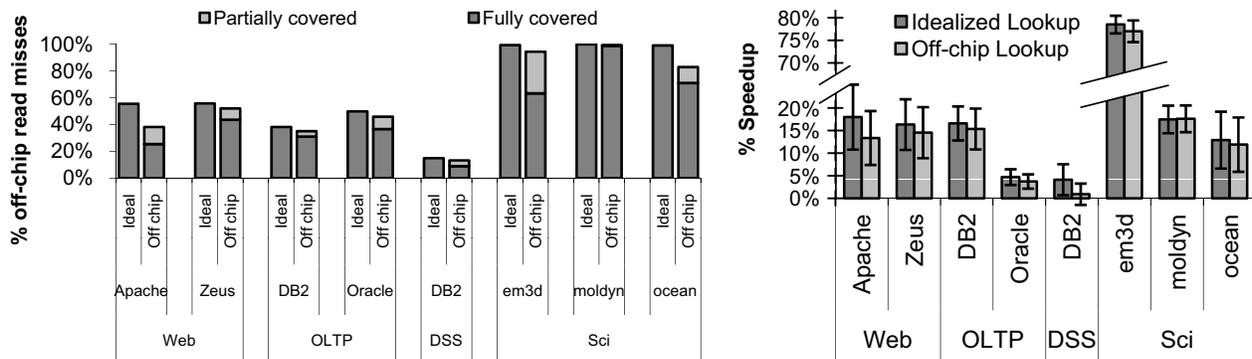
**FIGURE 9: Performance.** The left graph compares the coverage of idealized temporal streaming (*ideal*) and a practical STMS design with off-chip lookup (*off-chip*). The right graph compares the performance of the two designs, relative to a design with stride prefetching only.
