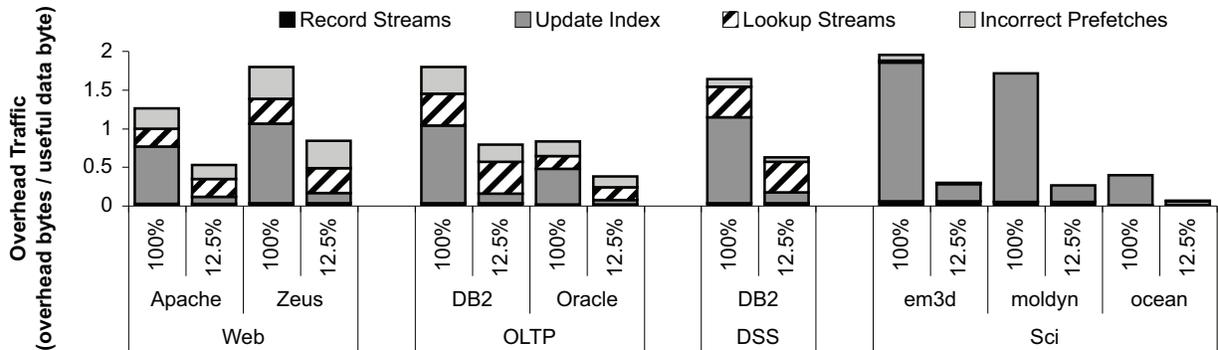
**FIGURE 7: Overhead traffic.** The left bar in each pair shows memory traffic overheads of off-chip index lookup without probabilistic update (sampling probability = 100%). The right bar shows overheads with a 12.5% probability.
