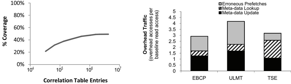
**FIGURE 1: Practicality challenges.** The left graph shows the number of correlation table entries required for a given coverage in commercial server workloads. One million correlation table entries can require up to 64MB of storage [6]. The right graph shows the memory traffic overheads of existing designs based on their published results [6,23,27]
