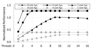
Fig. 5: Multicore prefetch-based access with various latencies. The values are normalized to the single-threaded on-demand DRAM baseline.
