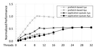
Fig. 7: Comparison of the application-managed queues and prefetch-based accesses with 1µs and 4µs device latencies.
