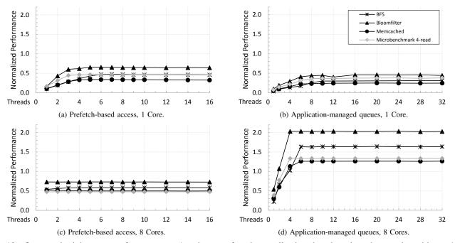
Fig. 10: One- and eight-core performance at 1µs latency for the application benchmarks, shown alongside a 4-read microbenchmark for comparison.
