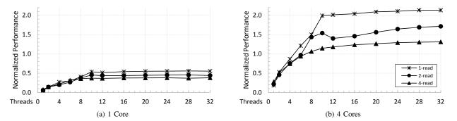
Fig. 9: Impact of MLP on software-managed queues with one and four cores. Each line is normalized to the corresponding DRAM baseline.
