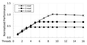
Fig. 6: 1µs prefetch-based access at various levels of MLP. Each line is normalized to the corresponding DRAM baseline.
