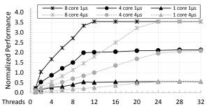
Fig. 8: Multicore comparison of software-managed queues with 1µs and 4µs device latencies.
