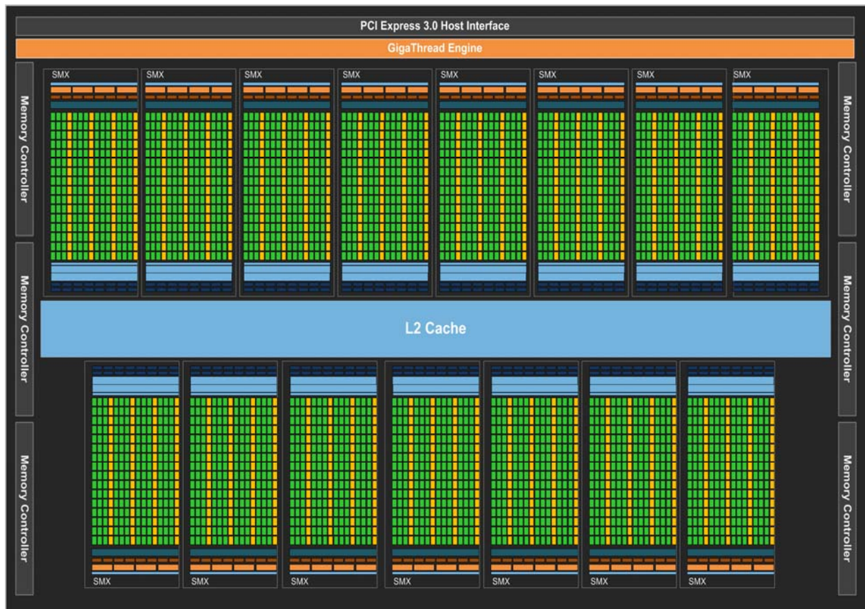
Kepler GK110 Full chip block diagram
