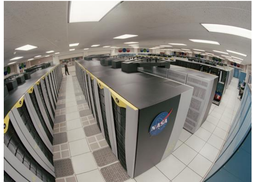
Columbia Supercomputer at NASA (Cluster of multi-rack 512-processor shared-memory machines)
