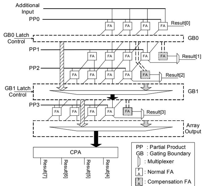
Figure 1. Structure of a 4x4 modified unsigned multiplier
