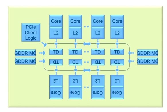
A multi-core chip with x86-based vector processors
