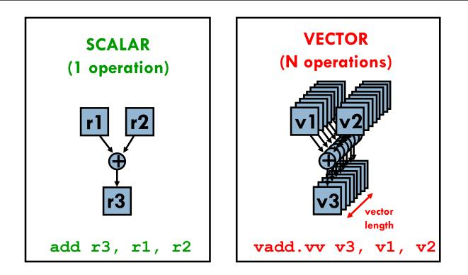
Scalar processors operate on single numbers (scalars)
