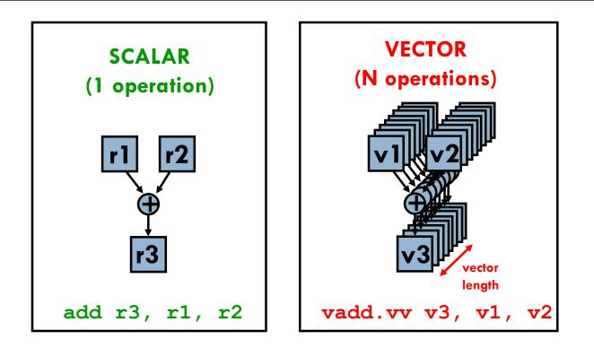
Scalar processors operate on single numbers (scalars)
